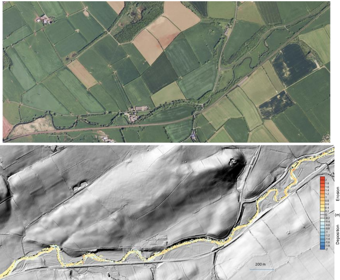
Figure 5. Orthophoto and DEM displaying measured morphologic change on the low gradient River Ellen active single thread study site. Flow direction is to the west.
